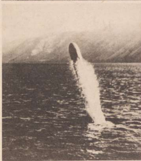
THIS Cruise Missile is said to be one of America's foremost 'war deterrents'. It can carry a nuclear warhead for 3,200km. to within 27m. of its target, flying just above ground level so that it is difficult to detect and destroy.
