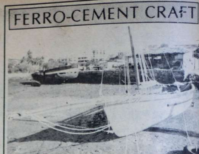
TOP: A ferro-cement boat rigged out as a simple yacht, and BELOW: A ferro-cement boat in formation, with the steel frame being carefully covered with layers of wire mesh, prior to being plastered with cement.
