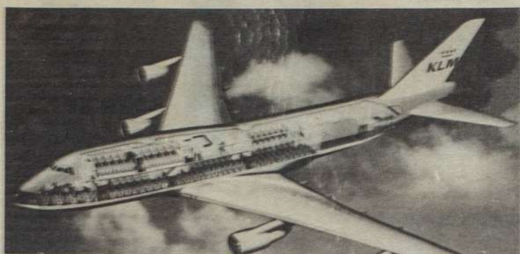
KLM's Boeing 747-300 with extended upper deck, fitted out in the new configuration.
