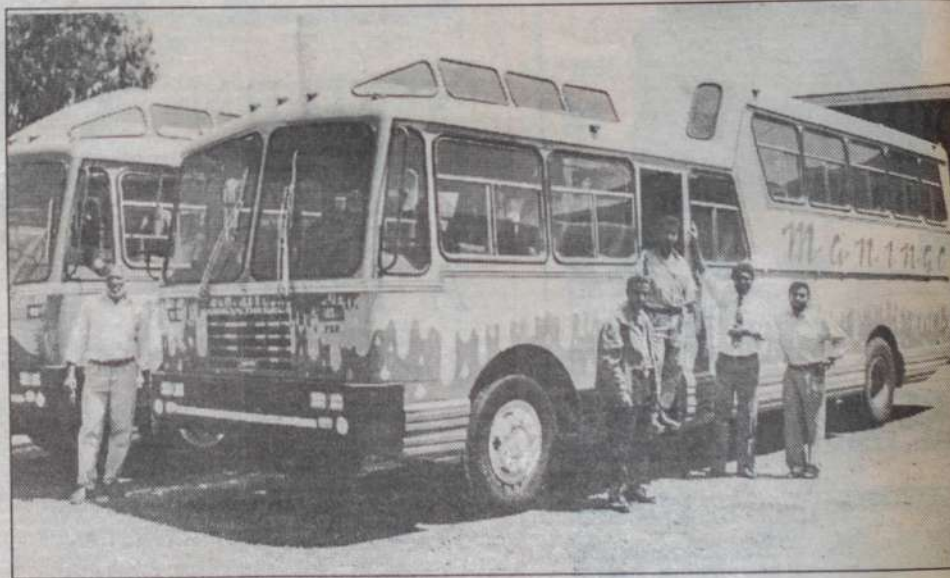
MANINGO TRANSPORTERS recently took delivery of four new Nissan Diesel CB 31 Coach buses from CMC Motors Group HCV Division. The buses in 2 x 2 configuration with high deck, have 46 reclining seats with head rests and ample luggage space. The buses will be in operation from Mombasa direct to Kampala and from Nairobi to Kampala. The Director of Maningo said, during the hand over, that passengers can be assured of a comfortable journey for the long distances. FROM LEFT - MR. Bical Ngotho, driver of one of the new Nissan Diesel CB 31 coach buses, Mr. Riadh Abdul, Mr. Dean Abdul, Directors, Maningo Transporters Ltd, Mr. Wilfred Munzyu, Sales Rep. HCV Division CMC Motors Group and Mr. Mahub Abdul, Director, Maningo Transporters, taking delivery of the new buses.
