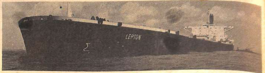
• THE V.L.C.C. M.T. Lepton seen off Dar es Salaam during the repairs on its condenser. This super tanker is 353 metres long, 55 metres wide and draws 22 metres draught. Its gross tonnage is 155,296, and deadweight 317,938 tons and is driven by turbines developing 36,000 s.h.p. PHOTOS: FLOYD LEMLEY (AP/WIDEWORLD)
