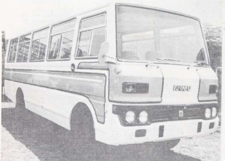
HOT SELLER — Seen here is the Isuzu 28 seater bus proving popular in the passenger conveyance business. Built on the TL53 Isuzu EB Chassis with a C240 diesel engine. This vehicle was recently displayed at the Kisumu
