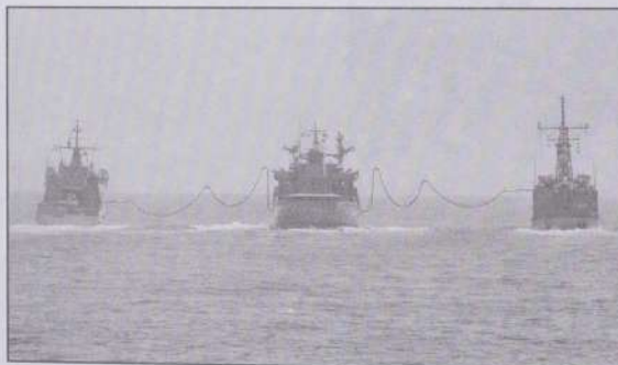
Replenishment tanker Rhön can supply two ships at a time.
