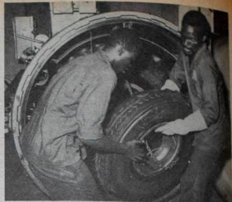
Employees of Car and General are pictured in the firms retread factory in Likoni Road, Mombasa removing a finished Bandag retread from the pressure chamber. Cold process retreads are now being made in Mombasa instead of sending casings to the Car and General factory in Nairobi for processing.
