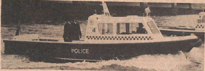
PERKINS POLICE PATROL BOAT — One of the latest Perkins marine-diesel Police Patrol boats selected for use by London's famous River Thames constabulary. The boats achieve upto 18 knots from the Perkins T6.3544 (M) Range, with four engines installed. Perkins, one of the U.K.'s largest manufacturers of marine diesel engines, celebrated its 50 years in the marine business last year. The new Police Patrol boats have caused considered 'export' interest from overseas.
