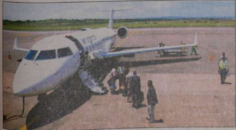
Air Uganda operates three aircraft in its fleet, with two 99 seat MD87s in a business and economy class configuration and one Bombardier CRJ-100 [seen above] in a 50 seat one class layout.
