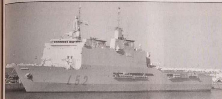
Castilla (L52) is a 13,000 tonnes Galicia-class landing platform dock (LPD), and is the twelfth ship of this name. She is the sister ship to the amphibious warfare vessel Galicia .
